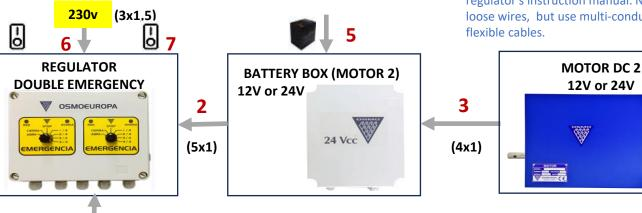
\* Refer to the wiring diagram in the regulator's instruction manual. Never use loose wires, but use multi-conductor
